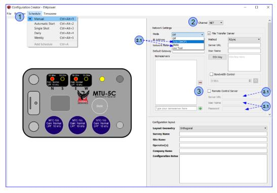
\*Configure recording details as desired (gains, filters, etc) and Save the configuration file to SD card
